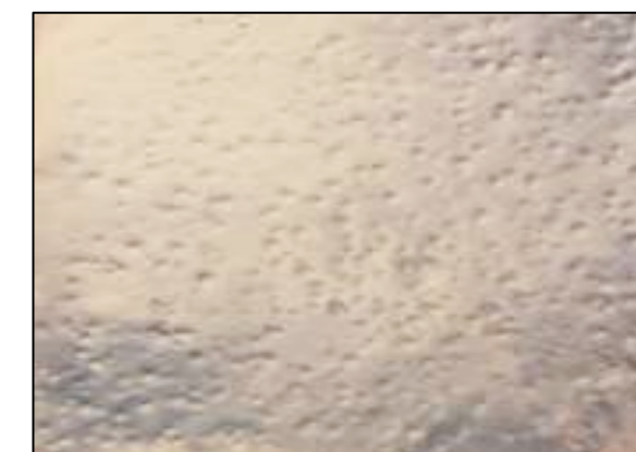
Image of the blows to the aluminum plate installed for the test.
